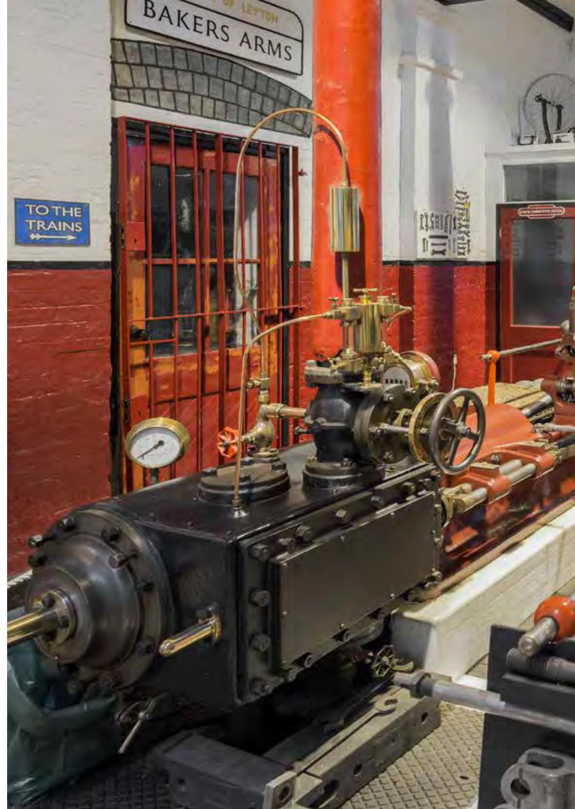
One of the Marshall 'C' Class horizontal steam engines, installed in 1897
